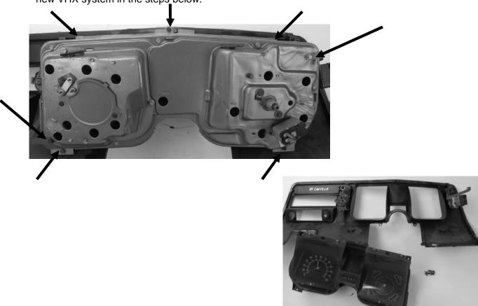
3. Remove the stock gauges from the stock lens spacer. The lens spacer is going to be reused to secure the new VHX gauges to the dash/bezel. Remove seven screws holding the gauges to the spacer. Save the screws, they will be reused to attach the new VHX system.
