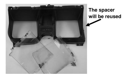
5. This step is optional for automatic transmission bezels only. If you purchased a separate GSS-2000 kit from Dakota Digital, the gear position can be displayed in the VHX message centers, therefore the stock gear position indicator can be removed.
