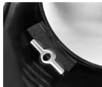
On the top two locations, fold the foam over the edges and make sure its not sticking into the visible window. In the bottom two corners, the area for the tape is slightly narrower than the foam so you will need to ensure the foam is curved with the opening in the housing.
