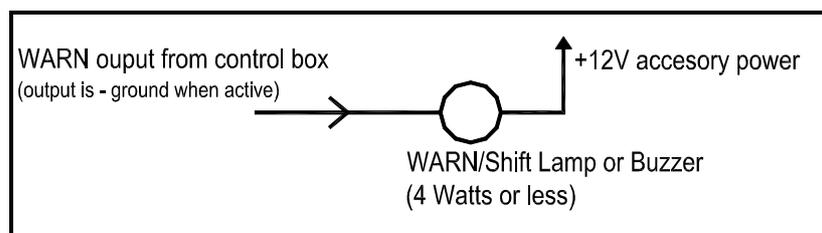
If you need the warn output to be “active high” or provide a +12V voltage to power something larger than 4wattt, a standard 12V relay can be used to accomplish this.
