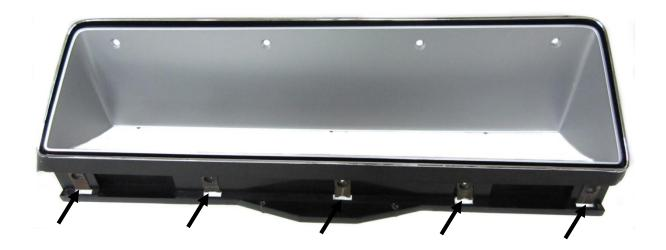
4. Place the Dakota Digital system into the bezel, taking care to align all mounting holes. Using the seven (7) provided #6-20x1-1/4" screws and washers, secure the gauges to the bezel. Pay special attention to align all visible surfaces before tightening the provided hardware. Some bezels may be bowed and not perfectly straight, requiring slight adjustments.
