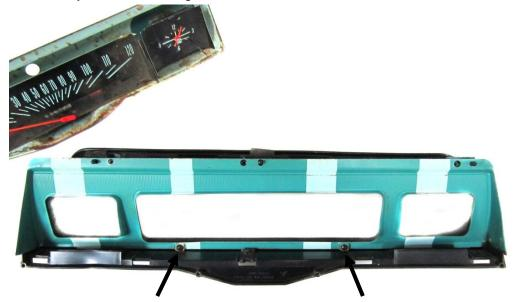
3. If using a reproduction bezel, be sure to keep the top four (4) mounting screws and five (5) factory clips (arrows below) from the factory gauge cluster as they will be used by the Dakota Digital system.
