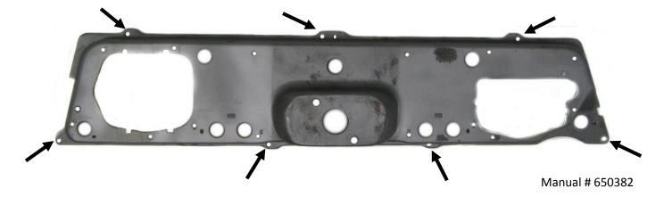
2. Remove the protective tape from the clear lens and install the VHX system into the bezel. Watch carefully as you insert the system so you don't scratch or damage the lens. The VHX system should align tightly, and the lens should sit flush with the bezel. Some reproduction bezels may require modification on the top side for the holes to line up properly.
