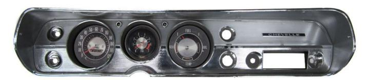
2. Remove the stock gauge, and lens from the bezel. The only items to be reused are the original front bezel and the four screws securing the gauges to the bezel; the other pieces can be discarded. Now is a good time to clean the bezel and remove any dirt or old lens gasket material.
