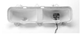
Feed the wires through the larger hole in the mounting plate. Guide the mounting plate to the bottom of the housing. The flat side of the mounting plate should be down and the side with the slight raised center should go up into the housing. This will align the mount in the original housing.
