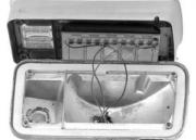
10. Fasten the lens back on with the four original screws.
