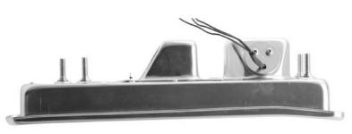
10. Place the original lens gasket into place and replace the tail light lens. Tighten the screws down carefully.
