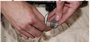
8. Now hold the LED assembly centered over the hole where the original bulb was and align the mounting plate from the bottom with the slot in the housing. The screw holes on the LED assembly and the mounting plate should be lined up.
