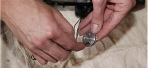
8. Now hold the LED assembly so that it is centered over the hole where the original bulb was located and align the mounting plate from the bottom with the slot in the housing. The screw holes should be lined up.
