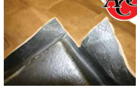
Mass-Backed Carpet shown which offer factory installed sound deadening material built in.
